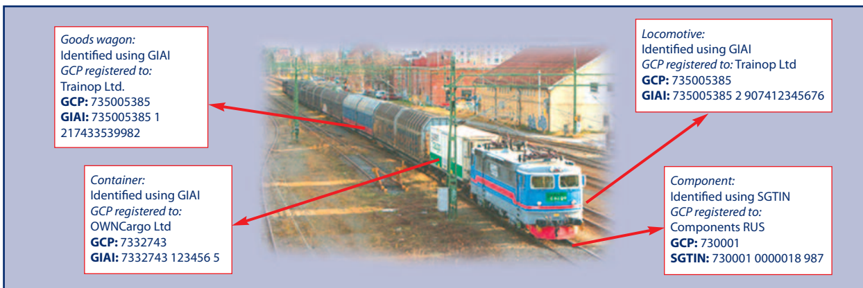
Illustration 3: The GS1 System has different identification keys for different purposes. The GS1 Company Prefix (GCP) forms a core part of the GS1 Keys to provide a way for GS1 users to uniquely and globally identify different things.
